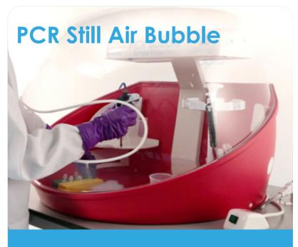
The PCR Still Air Bubble provides a comfortable to use, easy to clean enclosed environment for the preparation of PCR reagents.
